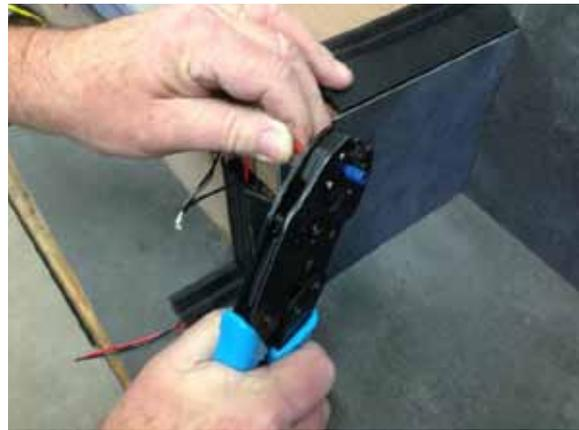
20. Crimp wires using correct size crimps.
