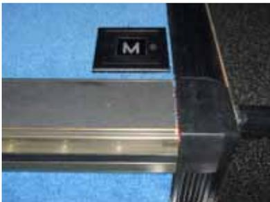
10. The crimped connectors should be inserted into the cable management, and the endcap fixed into the step edging
