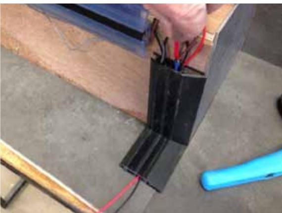
21. Insert crimps into cable management system.
