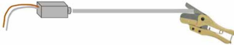
4. Fit ACP6/FR continuity rod into LEDASSY. Fit tube over rod and LEDASSY lug, then fit LEDASSY blank onto end of rod and tube
