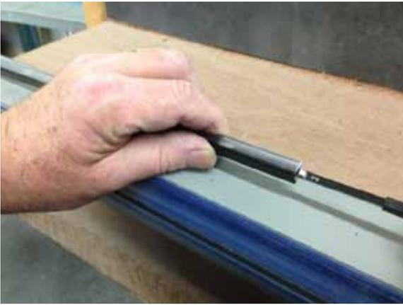
17. Insert lighting circuit (making sure black out strip is in the correct position).
