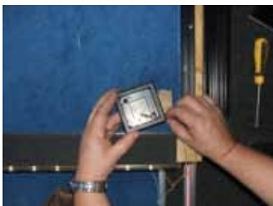
4. Pull the IAV led strip through the nearest cut out on the corner of the row indicator base
